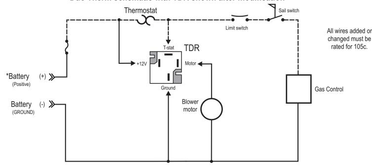
Note: Dashed lines indicate the thermostat control path
