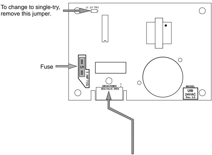
If this LED does not light up green, then check: LIMIT SWITCH SAIL SWITCH 5 AMP FUSE (on circuit board)
