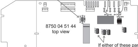
If either of these parts are discolored or blown, check wires to the gas valve for shorts to ground NOTE: Reversing the thermostat and gas valve wires will cause the same problem and so will plugging the gas valve wires into the wrong row.
